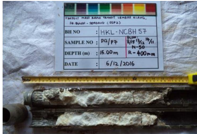
Figure 5. Typical weathered quartz obtained in SPT split spoon (Boon et al., 2023).
