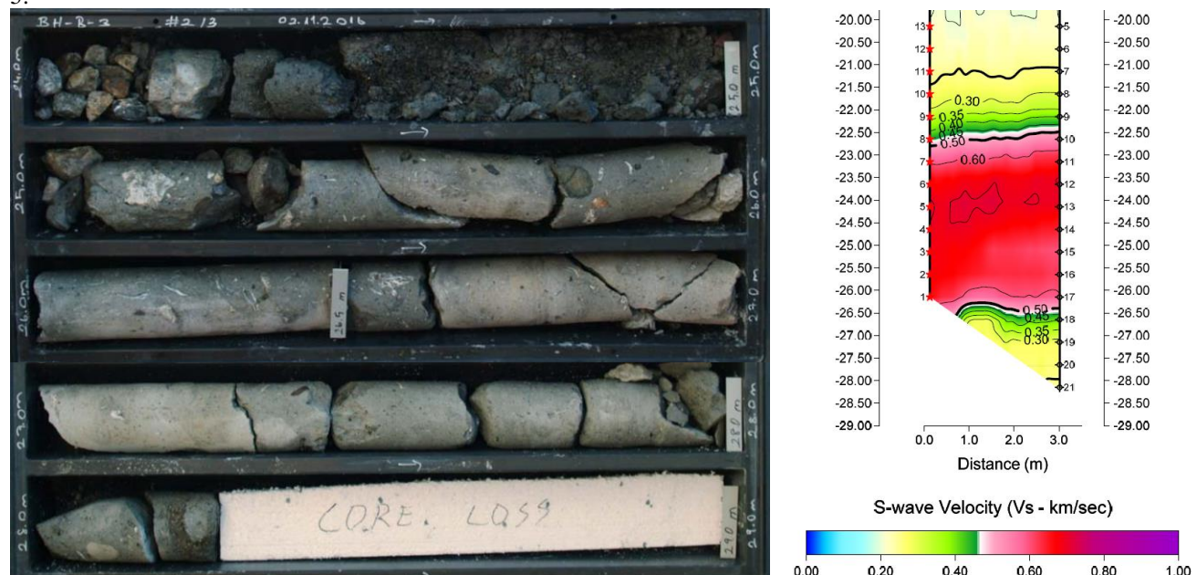
Figure 25. Core box photos of coring BH-B-3 between 24 and 29 m depth. Measured V_s across overlapping columns.
