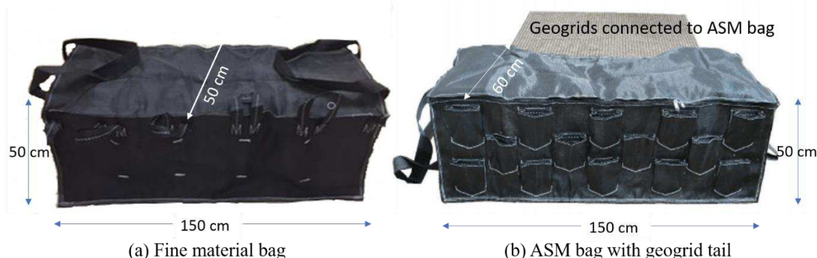
Figure 2. Geotextile bags for fine material and ASM.
