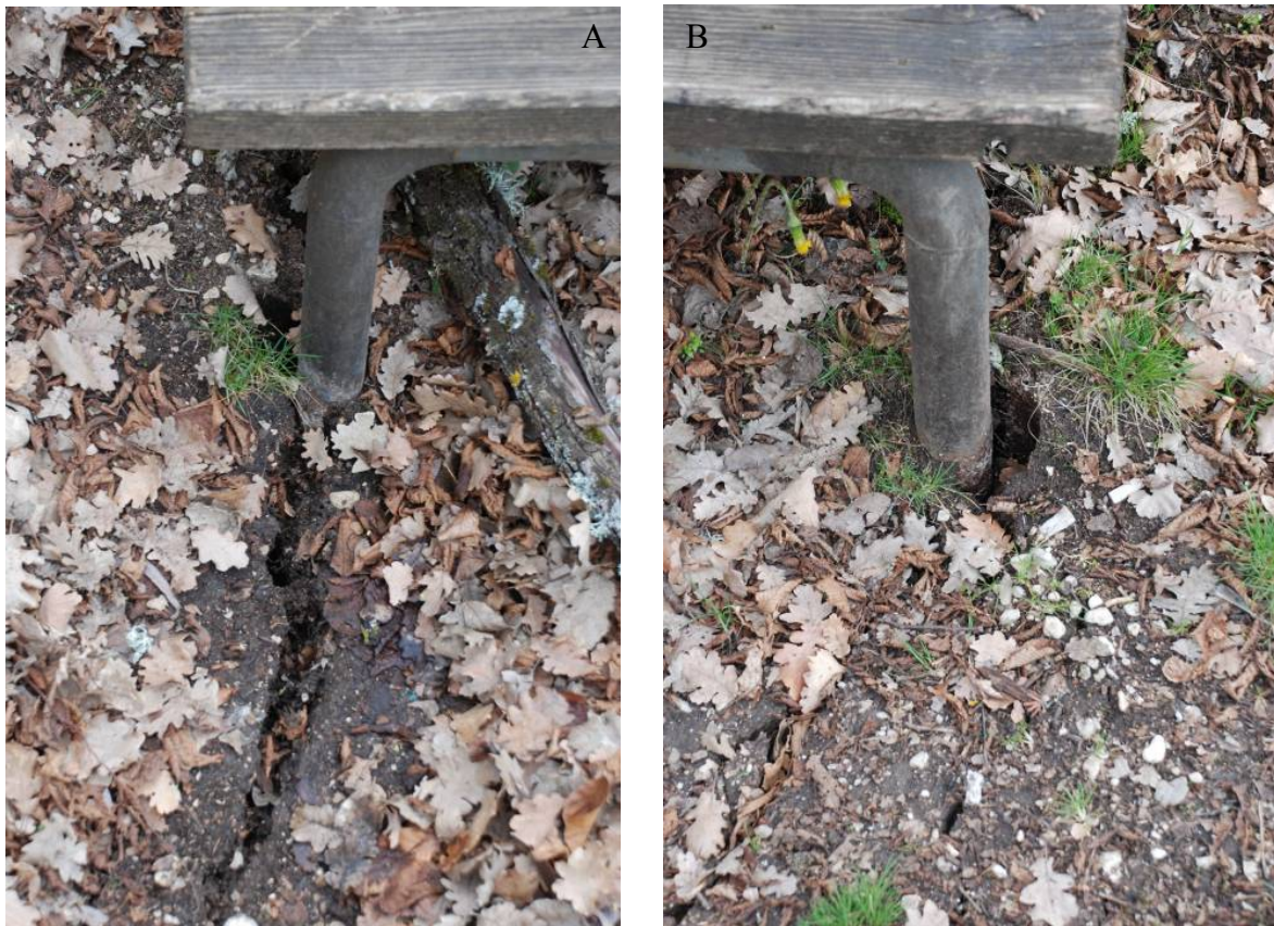
Figure 167. Characteristic deformations associated with the corners of the park bench at WP 31. (A) corner C2, (B) corner C3.
